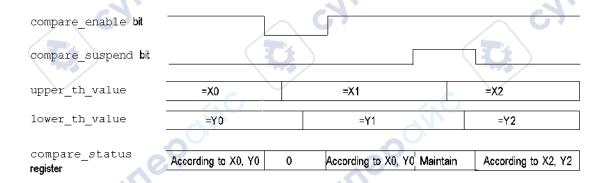
When the **compare enable bit** is false, the **compare status register** is cleared.
